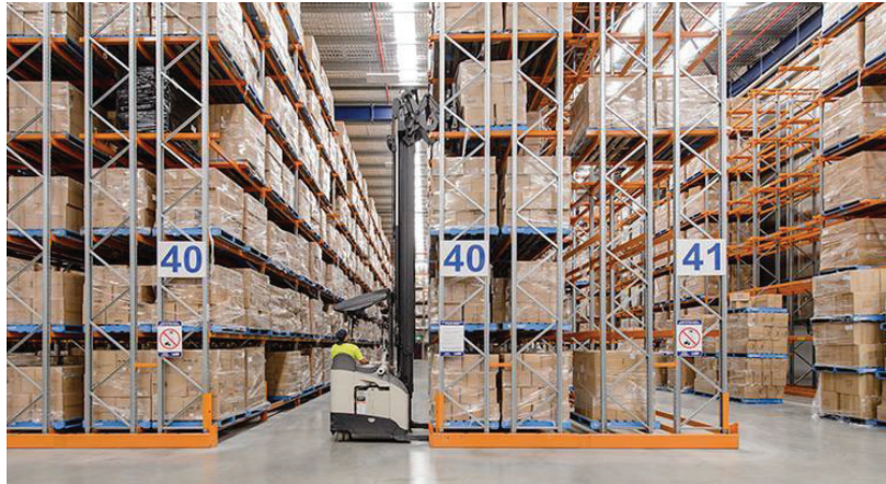
Figure 18 : Entreposage de type "double-deep"
